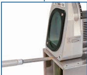
Precise adjustment of the electrode's stick-out.
